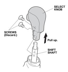
5. Install the new select knob with new screws. Using a torque screwdriver, torque the screws to 1.57 N·m (1.2 lbf·ft). Do not overtighten the screws.
