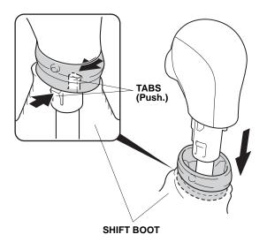
3. Pry on the bottom of the select knob cover and remove the cover.
