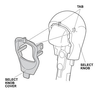
4. Remove the two screws from the select knob. Remove the select knob by pulling it up.
