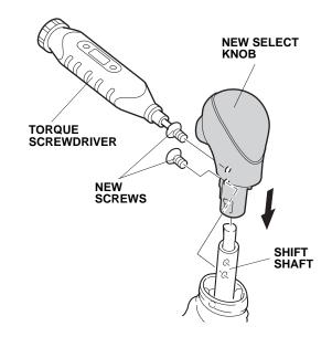
6. Install the select knob cover on the new select knob. NOTE: Make sure the cover is properly seated.
